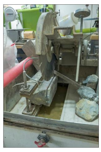
Once the rockhounding is done, and the stones are ready to be worked, several special tools are necessary. Here is an image of our 14" drop saw, which is used to cut large stones into smaller pieces suitable for working into finished pieces.
