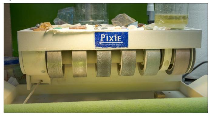
There are other types of saws that are used to cut the output from a saw like this into smaller pieces that are ready to be worked into a final piece. Shaping a cabochon usually requires the use of diamond-impregnated grinding wheels. The Pixie, shown below, is a common tool that contains several wheels, with consecutively finer grit from left to right.
