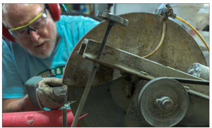
The blades on these saws, just like the blades of regular wood-cutting saws, require sharpening at intervals. Here I am sharpening the blade of this saw by tapping around the perimeter with the edge of a bastard file.
